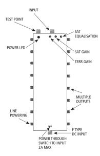
The Kingray Active Taps are specially designed for the distribution of terrestrial & satellite (Foxtel) services in a multiple dwelling application. They feature high output with adjustable gain and equalisation control.
