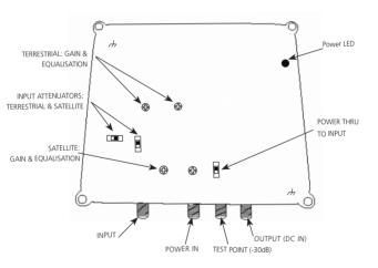
The Kingray DSB38F is a high gain Free-to-Air & Satellite distribution amplifier for use in SMATV applications. It features a combined single input & single output connector, with adjustable gain and equalisation controls, as well as input attenuators.
