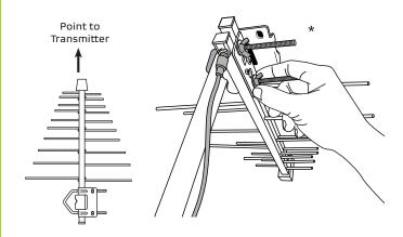
4. Point the antenna towards the transmitter. Tighten the wingnuts firmly once the antenna is positioned correctly.
