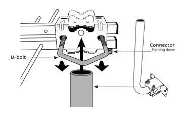
2. Slide the mast through the U-Bolt and finger tighten the wingnuts.
