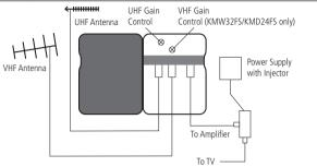
NOTE: There is a small switch located in between the input connectors underneath the sheilding. This will need to be switched to separate when two antennas are used. The left input should then be connected to the UHF antenna whilst the right input (middle connector) should be connected to the VHF antenna.
