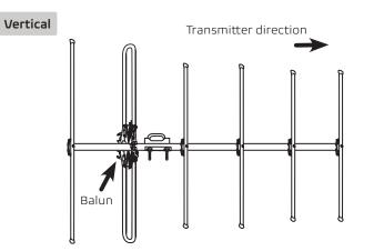
For vertical polarisation, remove the bracket and reattach to the boom so that the antenna can be mounted vertically.
