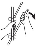
2 Attach loose elements to the boom as per the colour coding.
