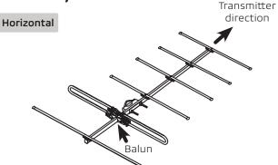
Make sure the balun is on the underside of the antenna and the antenna is pointing towards the transmitter.
