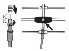
4 Loosen mounting bracket and attach to pole, tighten nuts with spanner.
