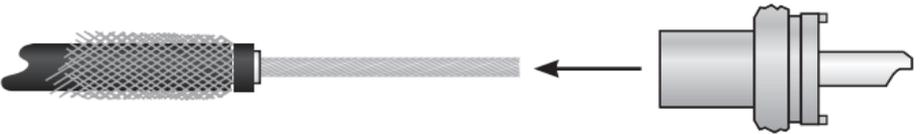
7. Trim off excess braid. Trim off excess and solder-exposed wire to pin.
