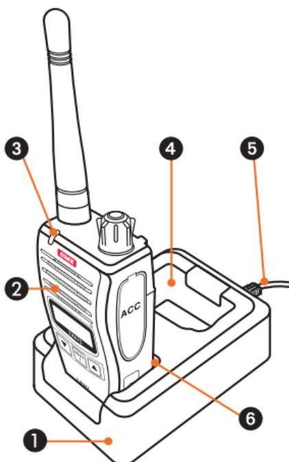
**\*NOTE:** When using the 12V vehicle charger to charge two radios via the dual desktop charger, we recommend switching both radios off while charging to ensure the batteries reach their full charge in the allotted 8 hour period. If one or more radios remain switched on during the charging cycle the batteries will achieve close to their full charge in the allotted time but the indicator LED may not switch to GREEN. This is due to the lower charge current available from the 12V vehicle charger.
